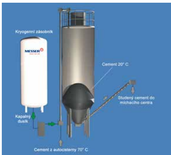
Obr. 3 - Princip technologie Cryoment-Flow
