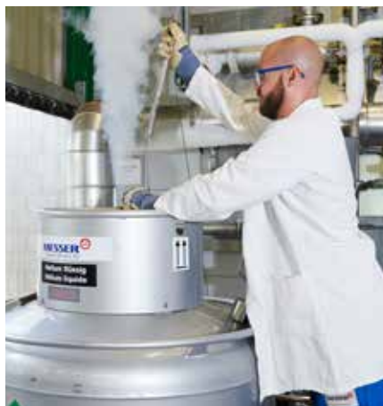
Depending on the quantities required, dewars ranging in size from 50 to 450 litres are available for the supply of helium.
