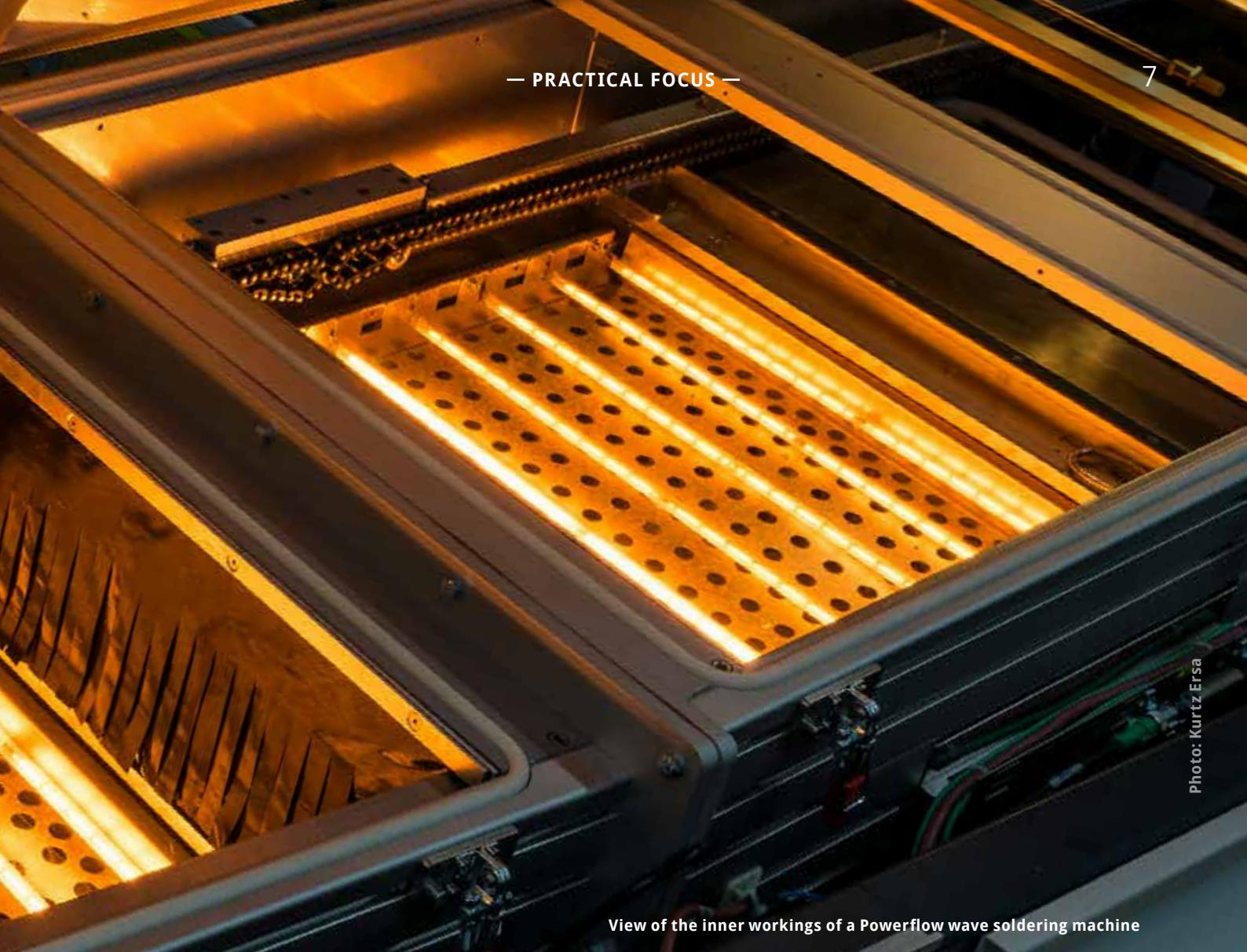
View of the inner workings of a Powerflow wave soldering machine
