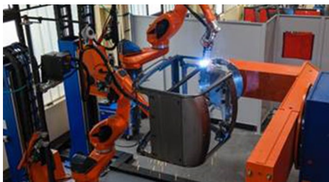
When welding the driver cabs, ternary mixtures ensure very smooth weld surfaces.
