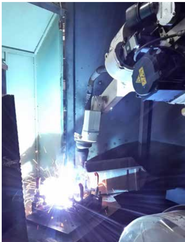
Mechanised MAG welding with Ferroline C18
