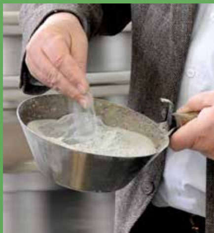
Cold grinding makes the PVC go brittle, allowing it to be ground to a fine powder.
