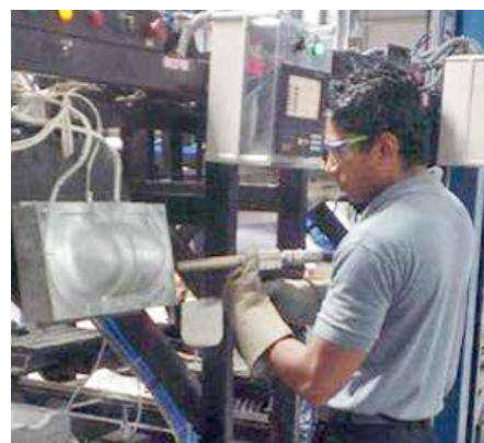
Dry ice blasting ensures gentle and efficient cleaning of the moulds used in the production of moulded foam cups.
