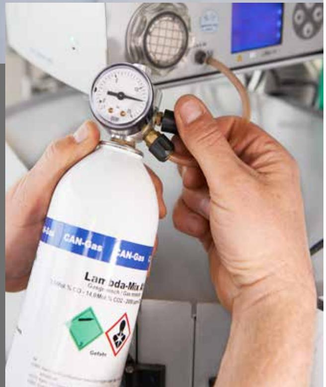
The exact exhaust gas values are then determined. Calibration gases such as Messer's Lambda-Mix guarantee the reliability of measurements.
