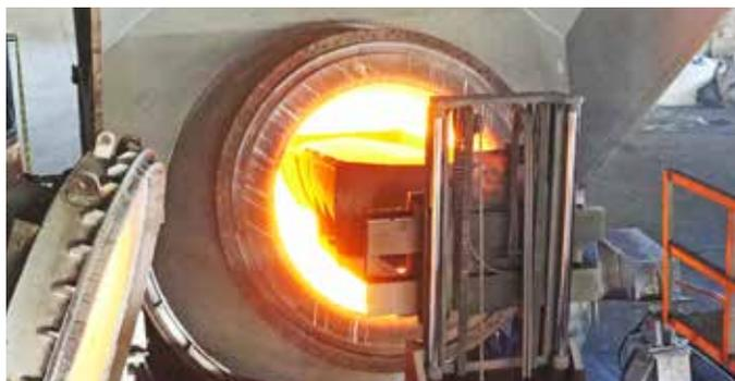
Furnace with oxy-fuel combustion system
