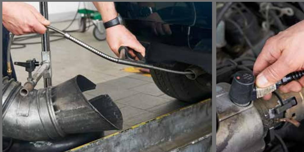
Cars need to undergo an exhaust emissions test every two years in Germany. This involves sensors being attached to the exhaust and the cylinder head.
