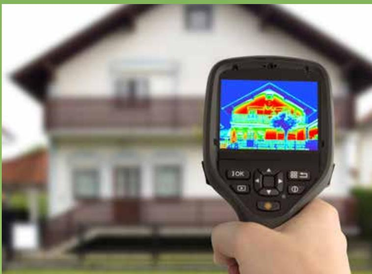
Thermal imaging cameras provide a visual representation of the heat losses from buildings and give a clear indication of where additional insulation is required.
