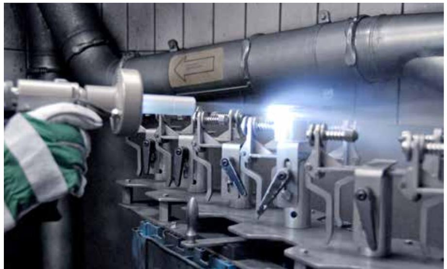
The gun light fitted to the gun illuminates the narrow annular groove during cleaning.
