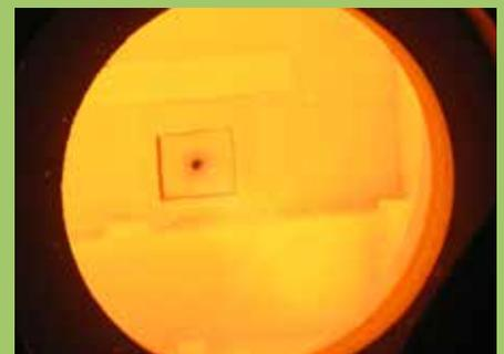
The “flameless” Oxipyr burner from Messer – being heated up (top) and at 1,550 degrees Celsius (bottom) – achieves maximum combustion efficiency with pure oxygen.
