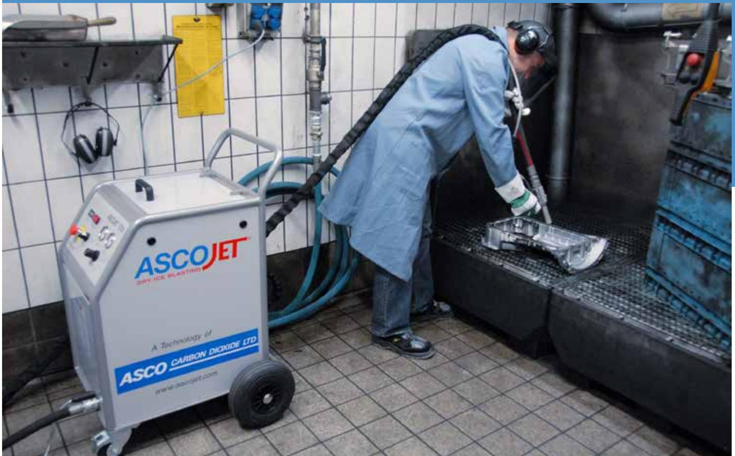
Cleaning an engine component with dry ice blasting technology from ASCO Carbon Dioxide
