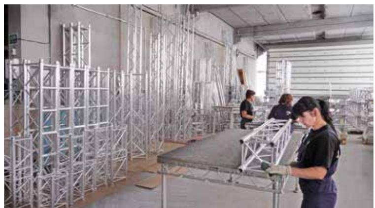
Final inspection of finished trussing systems
