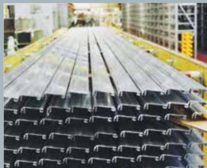
Founded in 1796 as a button and buckle factory, Gerhardi Alutechnik GmbH & Co. KG in Lüdenscheid has been family-owned for five generations. Using the company's two modern extruders, the 100 staff can transform 16,000 tonnes of aluminium billets into extruded profiles annually. The company sells its products to customers in a range of industries, including the machine-building, construction, automotive and electronics industries.
