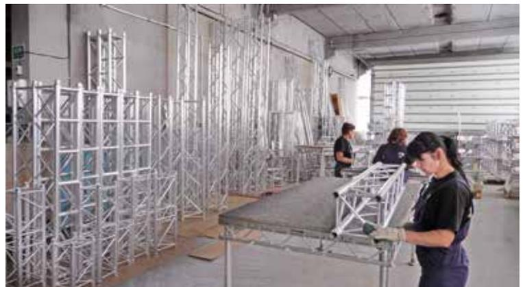
Final inspection of finished trussing systems
