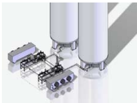
The complete solution: CO 2 dosing systems with tanks and atmospheric CO 2 vaporisers. The double line ensures a fully redundant system.
