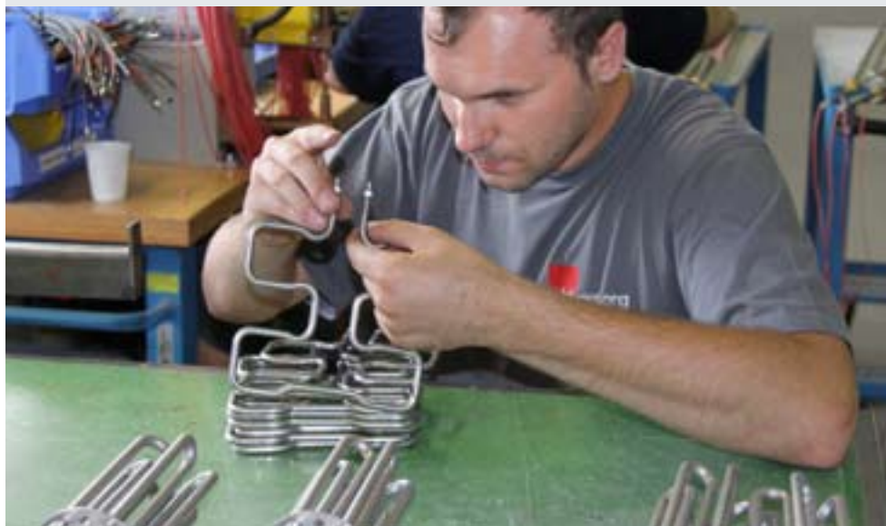
Stefan Cuturic screws together the cooled, manually bent heating elements.
