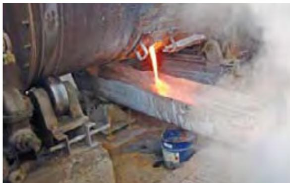
Oxypry-Plon burner for oxygen dosing in frit production
