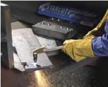
The STARCUT hand cutting torch for flame cutting material of up to 500 mm in thickness and for gouging
