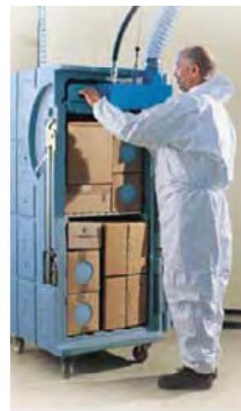
The top section of the Siber container is filled with dry ice snow.
