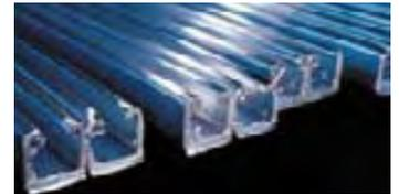
Nitrogen from Messer is used for cooling during aluminium extrusion.
